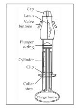
Figure 6: MVA Plus Aspirator
