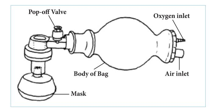
**Posterior part of bag** consists of two inlets. The wider inlet is for air and the other one for oxygen. Oxygen tubing is attached at the oxygen inlet and the oxygen reservoir, if used, is attached to the air inlet.
