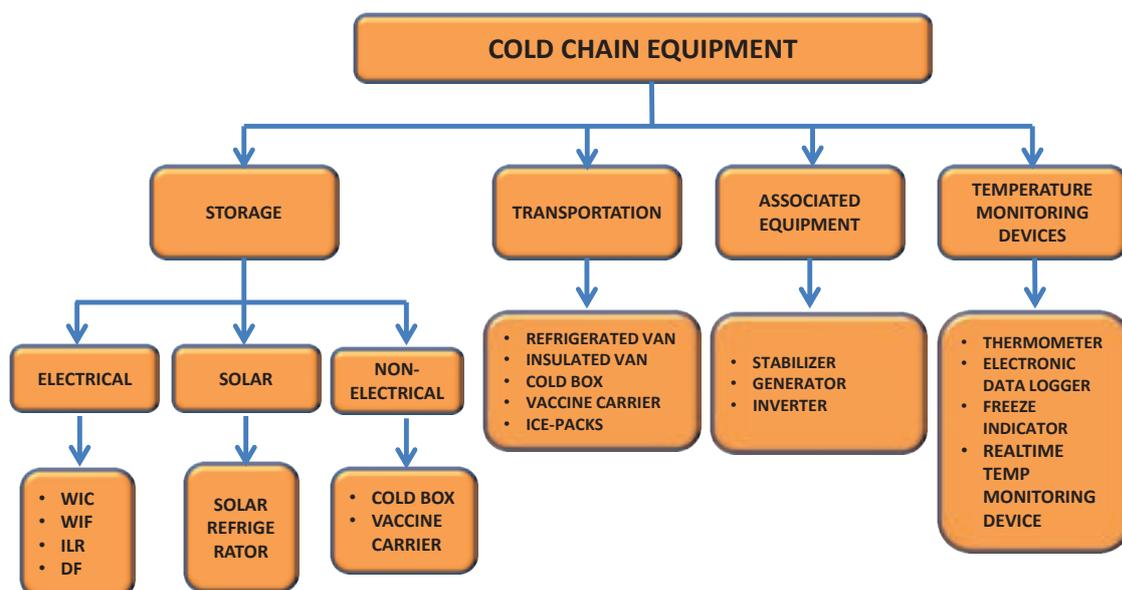
WIC – walk-in cooler; WIF – walk-in freezer; ILR – ice-lined refrigerator; DF – deep freezer
