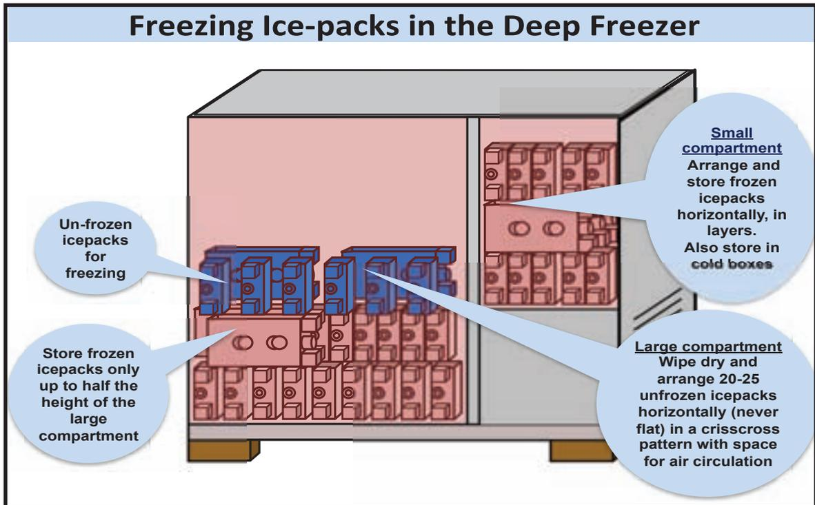
Fig. 4.6. Brick layered ice packs in deep freezer
