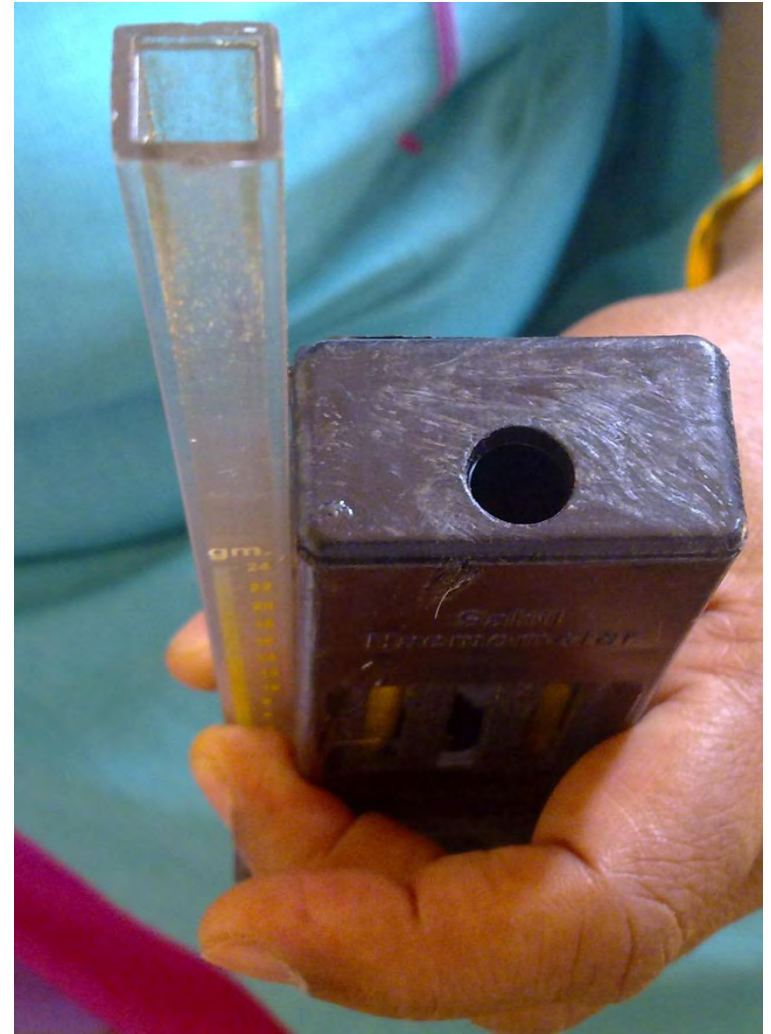
Haemoglobinometer with round hole and square glass tube
